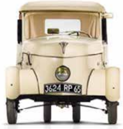
The PEUGEOT VLV Microcar Powered by four 12V batteries with a speed of 22 mph.
